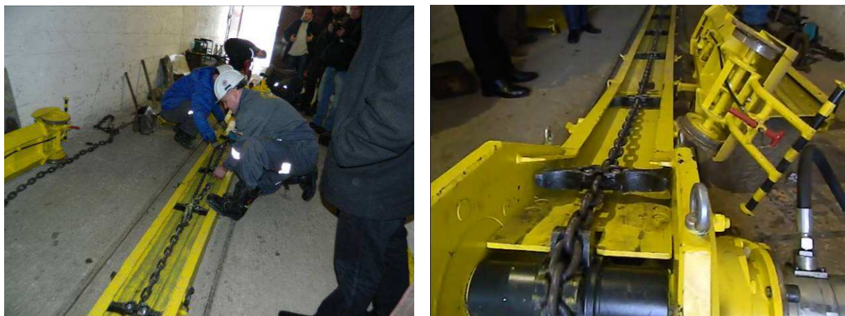
Fig. 14: Tests of the conveyor and its shuttle platform at CSRG
