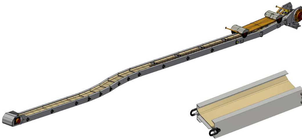
Fig.2: 3D model of the rescue conveyer with the shuttle platform and the new version of trough (by KOMAG)
