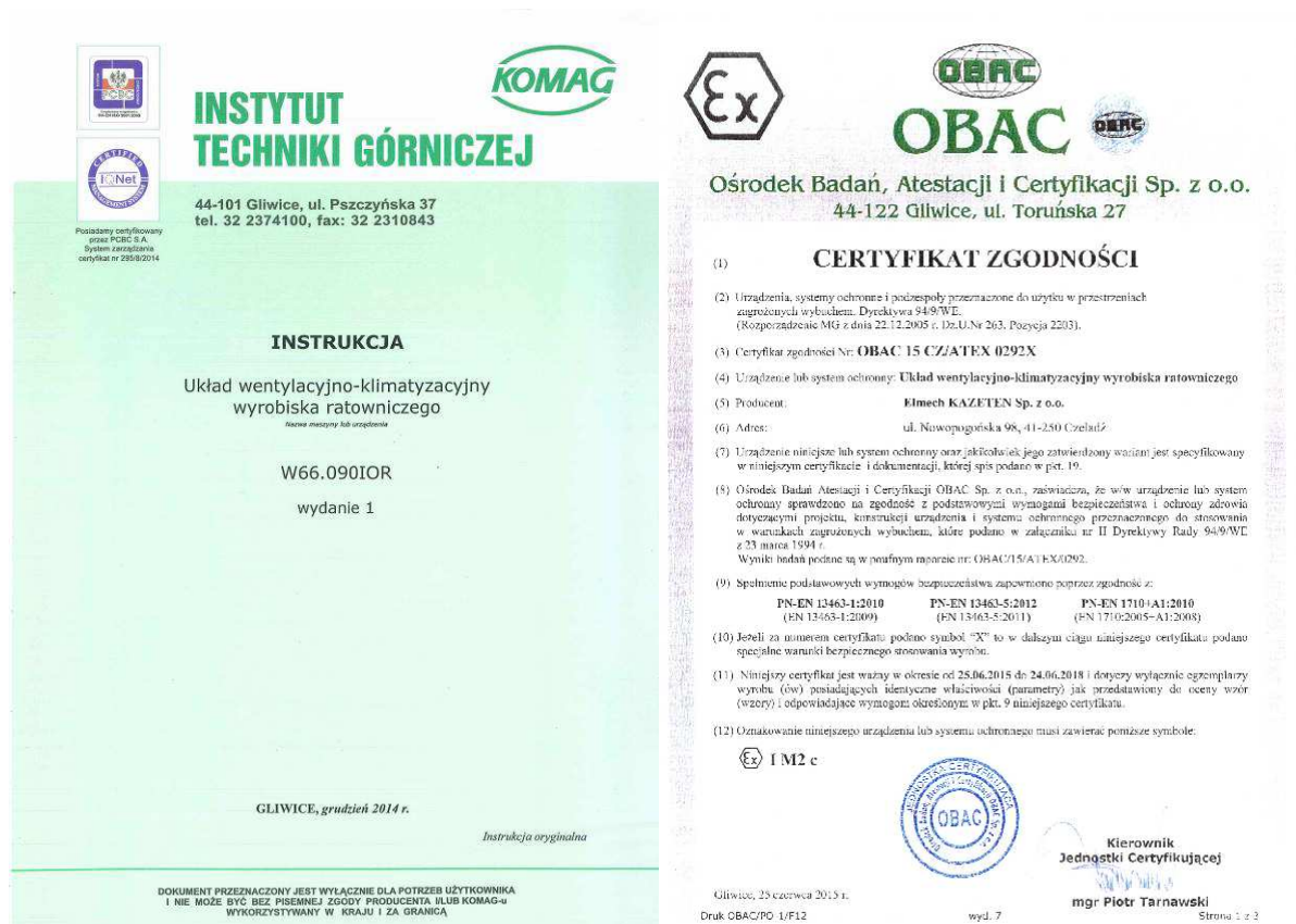
Fig.30: Technical manual of air conditioner and the certificate for conformity of air conditioner which confirms that product is classified for group I category M2 according to 94/9/WE Directive (ATEX)
