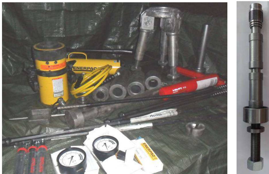
Fig.33. Components of UDWR-1 device (left) and the prototype of the bolt K-260 (right)
