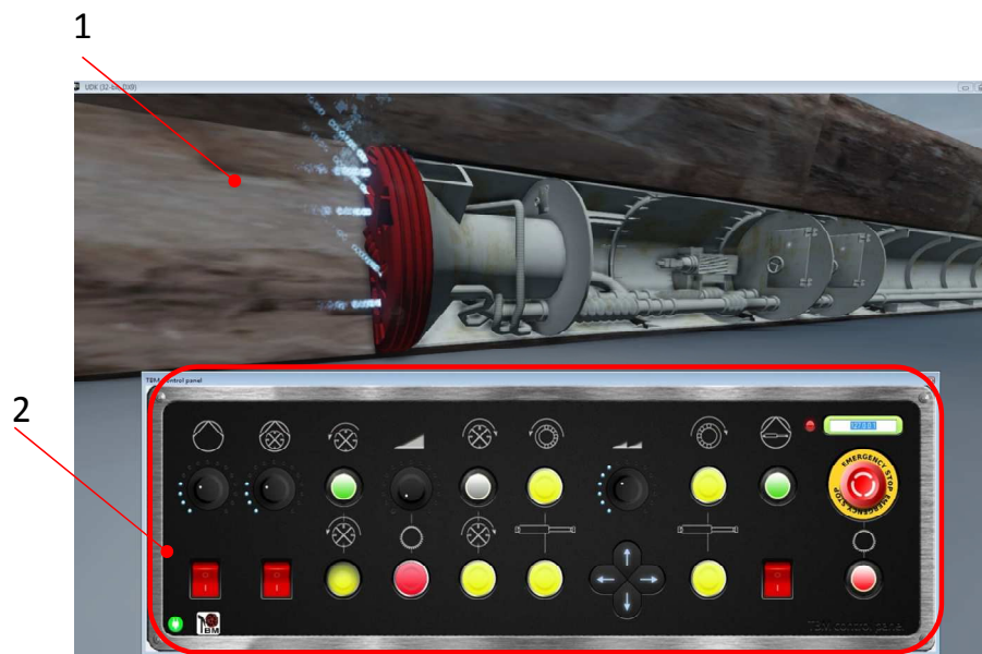
Fig. 88: Window of the application simulating the operation of boring machine
