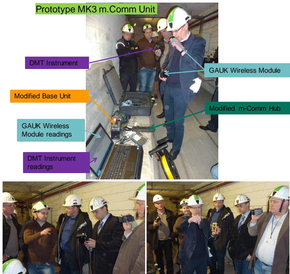
Fig. 63: Field trial of the MK3 prototype m-Comm at the CSRG training galleries
