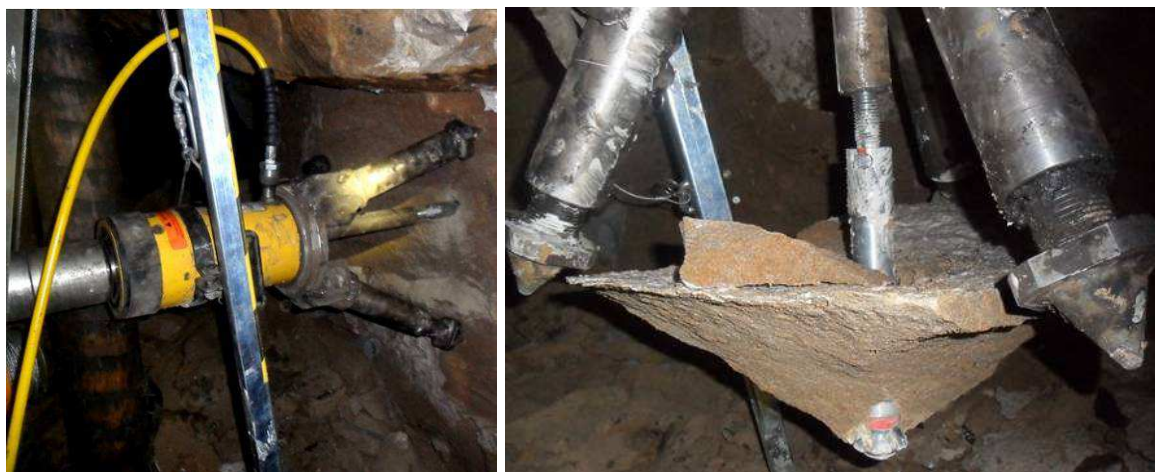
Fig.35. Detaching the rock solid with use of HDA-P bolt
