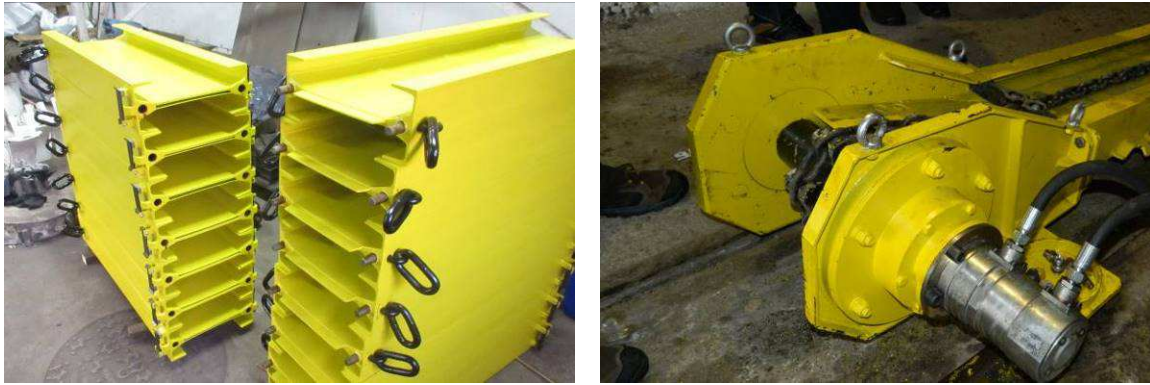
Fig.12: The new troughs (on the left) and conveyors drive (on the right)
