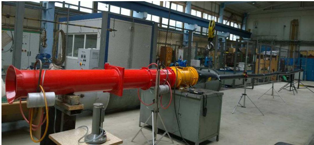
Fig.29: Testing the efficiency of air conditioner blower when air is supplied by ventube of diameter 120 mm
