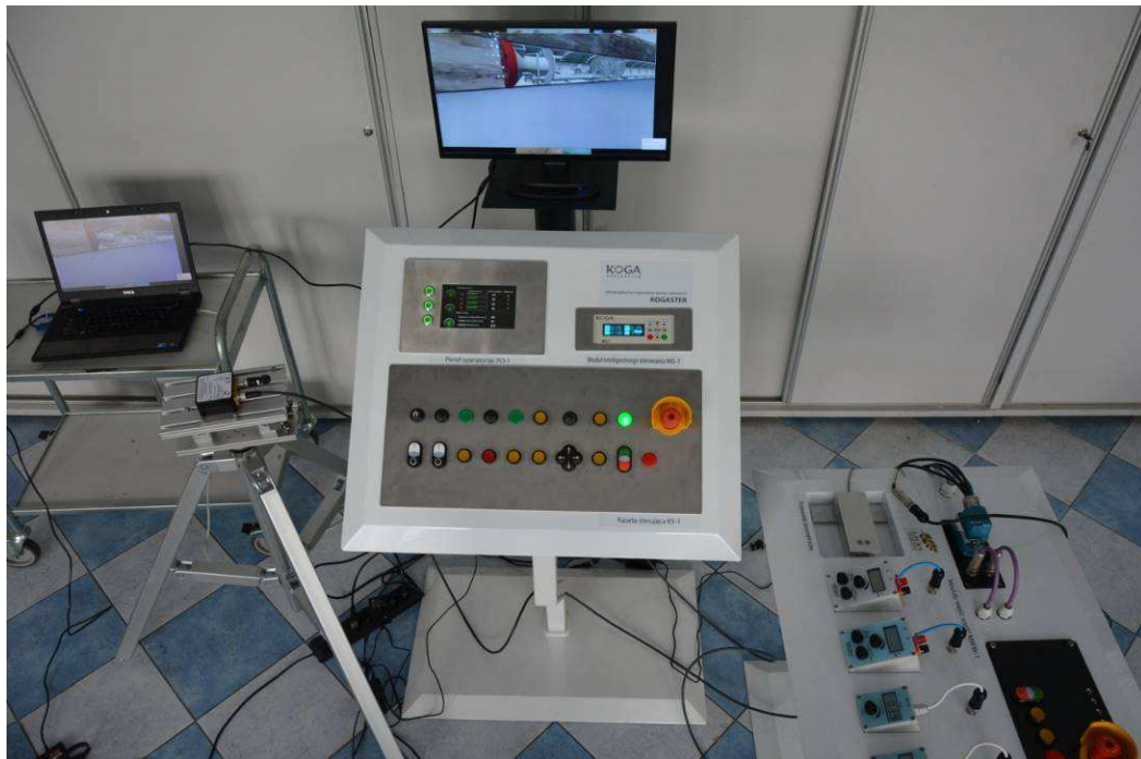
Fig. 42: System for simulation of boring machine control
