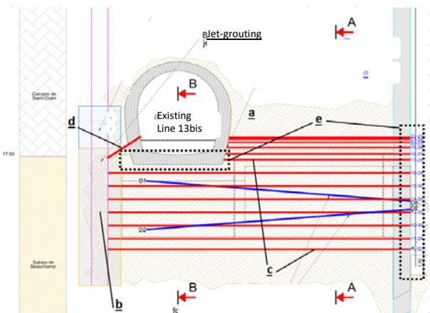
Fig. 2 Longitudinal profile of AGF intervention
