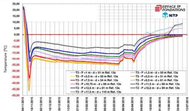
Fig. 5 Ground temperature vs time as detected by T-sensor T3
