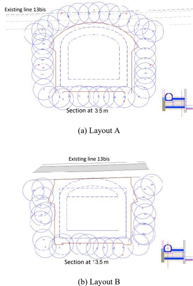
Fig. 3 As-built layout of freeze pipes – (a) Layout A, 3.5m from the shaft – (b) Layout B, 13.5m from the shaft TGI
