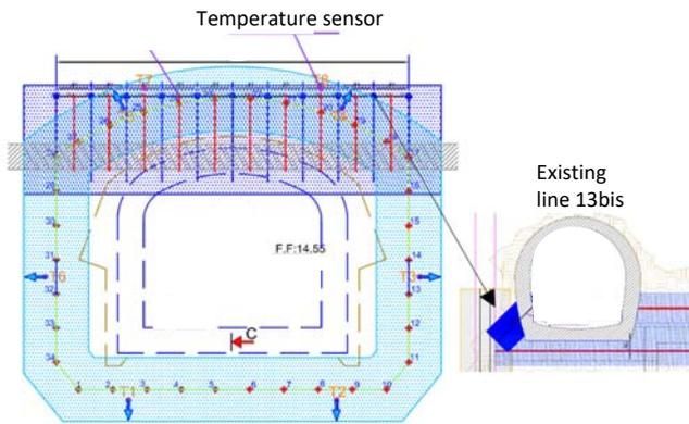
Fig. 4 Theoretical layout of freeze pipes – Layout C
