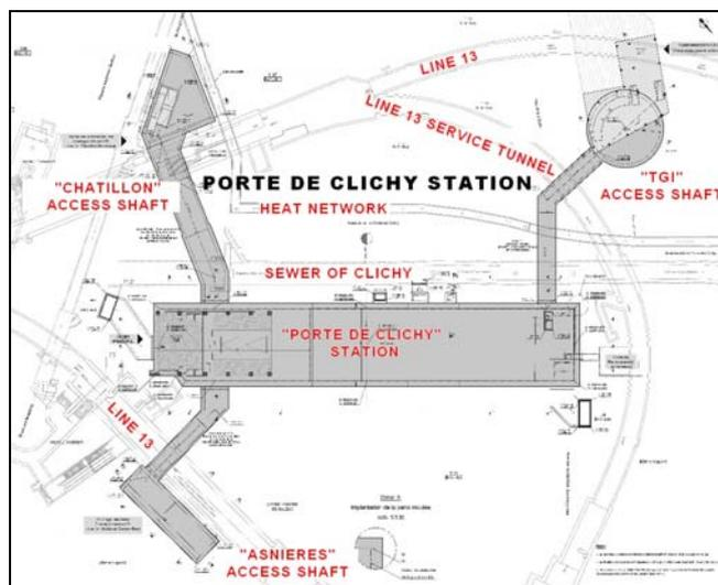
Fig. 1 Plan view of PCY station
