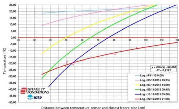
Fig. 7 Ground temperature vs distance between sensors and the closest freeze-pipe
