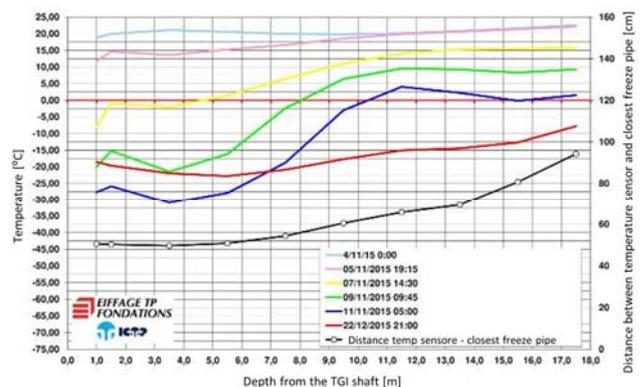
Fig. 6 Ground temperature vs depth
