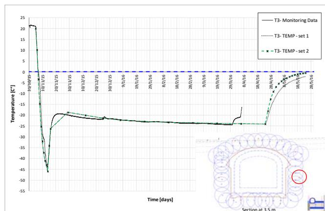
Fig. 11 Ground temperature vs time – back analyses results
