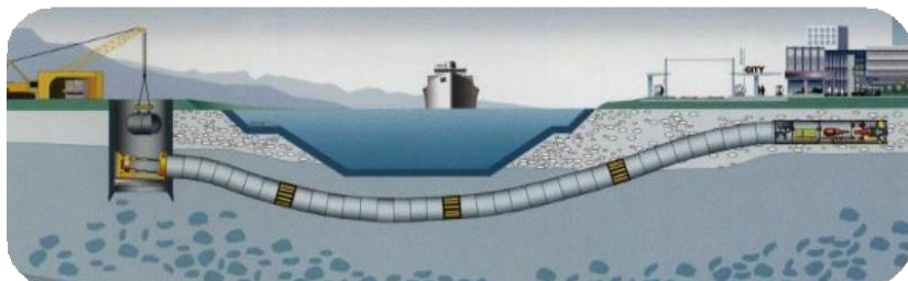
Microtunnel Application: River Crossing
