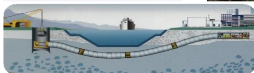
Microtunnel Application: River Crossing
